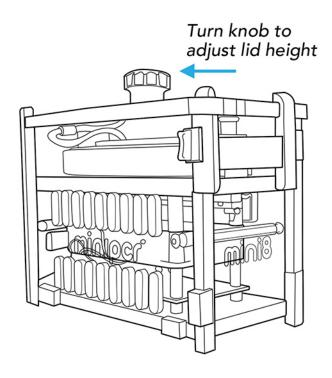
2. Adjust the height of the heated lid. Fully untwist (counterclockwise) the adjustment knob and press the lid down until the lid clicks shut. Tighten the adjustment knob (clockwise) until you feel light resistance from the tube caps. Be careful not to over-tighten.
