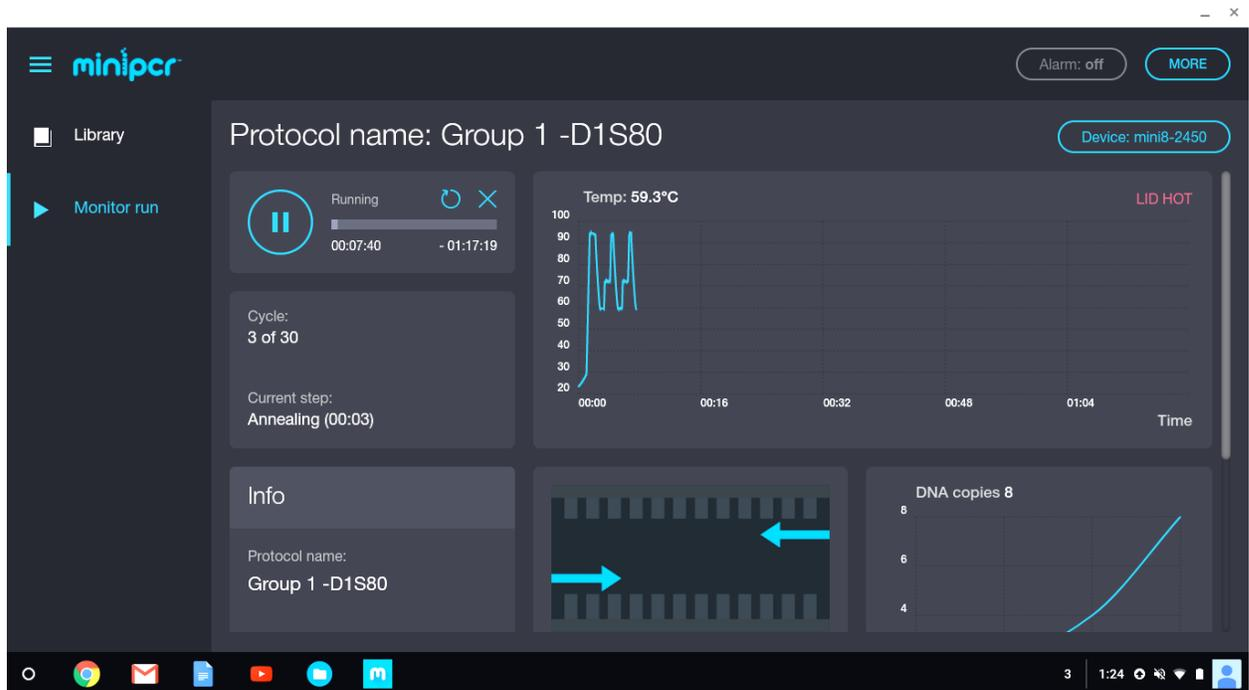
*The miniPCR™ software allows each lab group to monitor the reaction parameters in real time, and to export the reaction data for analysis as a spreadsheet.*
