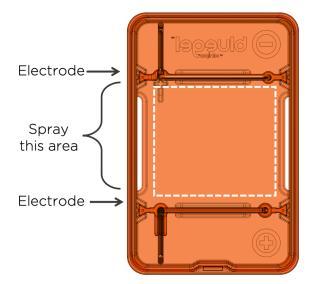
5. Place the orange cover on the blue base, matching the positive symbol on the orange cover with the positive symbol on the blue base.
